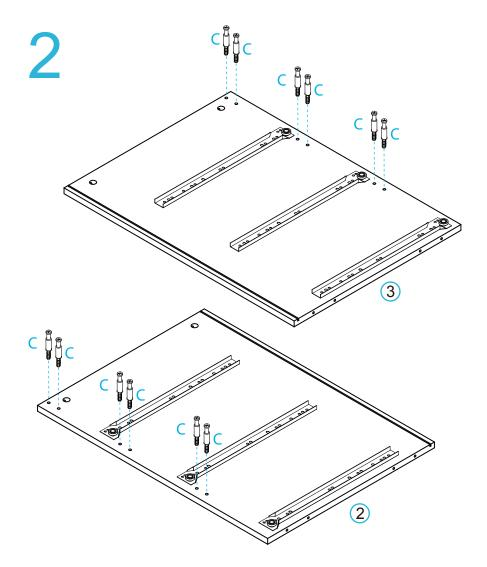
Insert 6x bolts (C) into panel [2]. Insert 6x bolts (C) into panel [3]. Tighten with a screwdriver.
