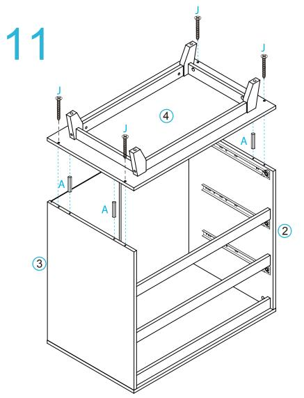
Insert 4x dowels (A) into the top of panel [2] and [3]. Attach the base panel [4] by inserting 4x long screws (J) and tighten with a screwdriver.
