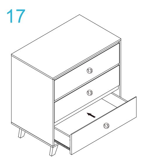
Insert the assembled drawers into the corresponding compartments as shown. Ensure the drawers slide easily along the rails.
