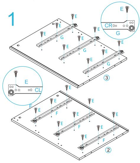
Attach 3xCL runner tracks (F) to panel [2] using 9x small screws (E). Attach 3xCR runner tracks (F) to panel [3] using 9x small screws (E). Tighten with a screwdriver.
