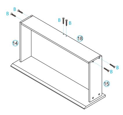
Attach panels [14], [15] and [18] as shown using 6x screws (B). Tighten with a screwdriver.
