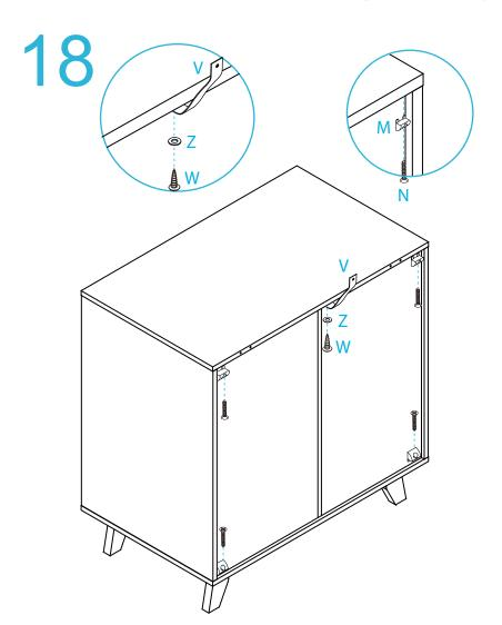
Attach 4x wedges (M) into the corners of the back of the unit and secure with 4x screws (N). Tighten with a screwdriver. Attach 1x safety strap (V) to the top of the back side of the unit as shown using 1x washer (Z) and 1x screw (W). Tighten with a screwdriver.
