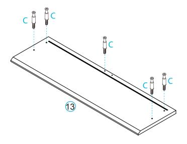
Insert 5x bolts (C) into panel [13]. Tighten with a screwdriver.
