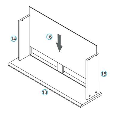
Insert dowel (A) into panel [13]. Attach panels [14], [15] and [17] to panel [13] secure with 5x locking nuts (D). Tighten with a screwdriver.
