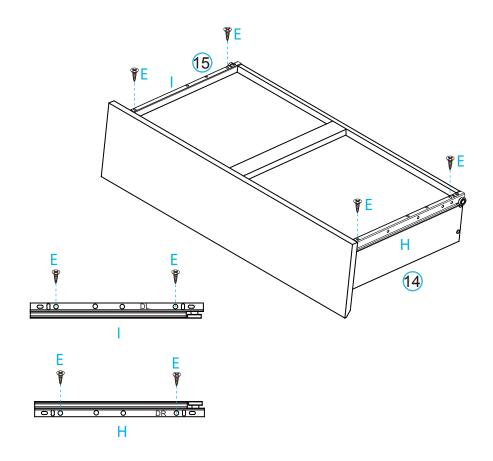
Attach slide rails (I) and slide rails (H) to the underside of the side panels as shown. Secure with 4x screws (E) and tighten with a screwdriver.
