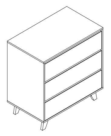
Once assembled lift furniture into place, do not drag. Use a drill to create a small hole lining up with the top of the safety strap (V). Fasten to wall using 1x washer (Z), 1x wall plug (X) and 1x screw (Y). Ensure unit is balanced and steady before use.
